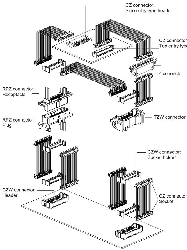
※ CZ connector used for the harness shown in the above-mentioned figure can be replaced to CZH connector.
