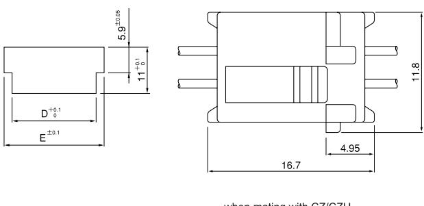
D,E dimensions: Refer to TZ connector (Until for wire-to-wire connection).
